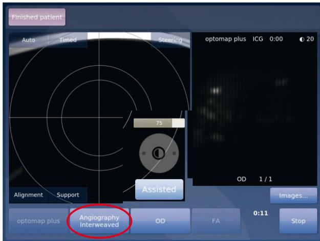
2. You may begin the session in Angiography Interweaved mode and change to Angiography mode without impacting the simultaneously running timers. This can be used to manually capture FA or ICG images. Switching to Angiography mode allows you to manually select either FA or ICG capture without the system automatically changing over.
