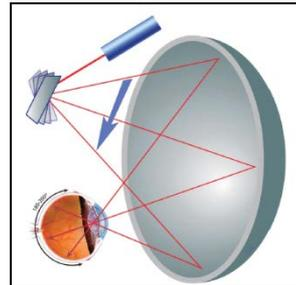
Schematic of UWF imaging using an ellipsoidal mirror. A laser light source is reflected off the galvanometer mirrors onto an ellipsoidal mirror. The second focal point of the mirror resides within the eye, which facilitates image acquisition anterior to the equator.
